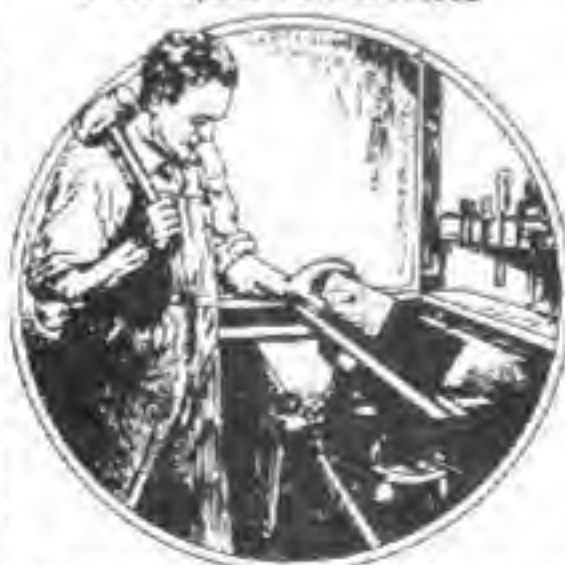
Sheet Metal Clamped in Vise to Bent by Means of Wooden Block and Mallet
